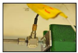
Figure 4.15. PCB Force Sensor
