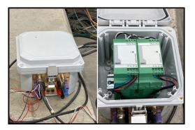
Figure 4.22. New LVDT Power Supply
